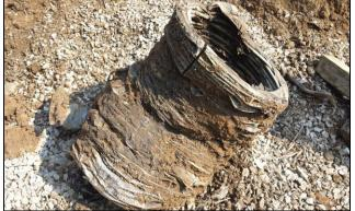
Figure 2. Compressed CMP
